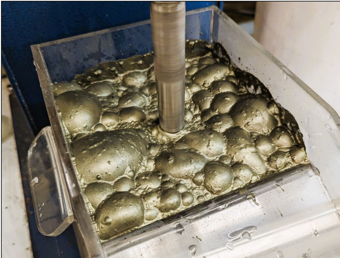
Figure 1. Rougher flotation test work.
